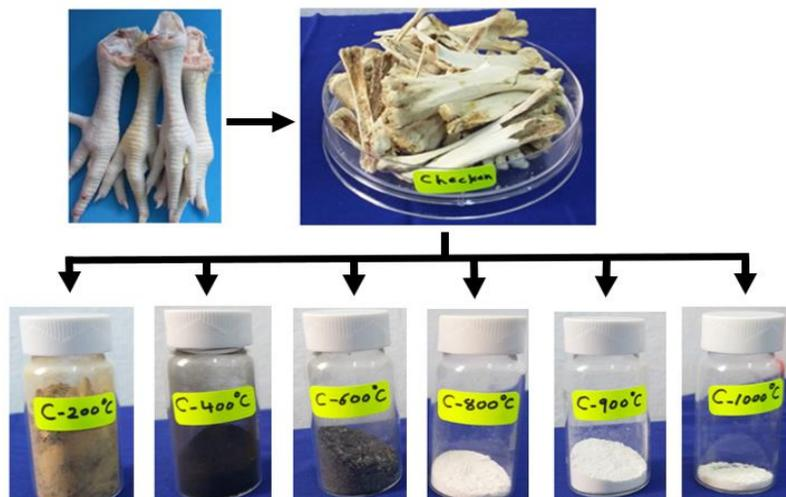
Fig.1. Shows the collected bones treated at different temperatures.
